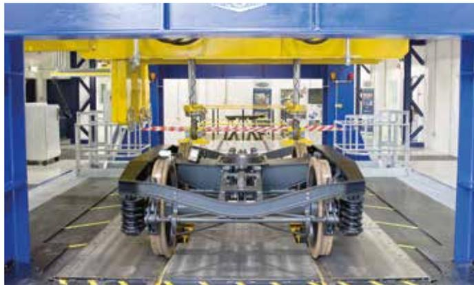
In the frame: a new £4.5 million 150-tonne bogie test rig at the IRR in Huddersfield. Tony Miles
